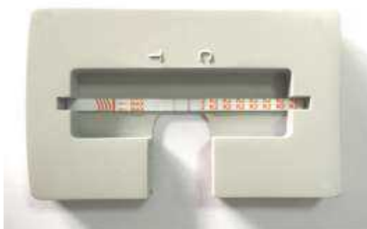
Fig.16 The placement of test strip in the cartridge
